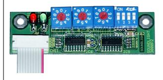
DMX Personality and DMX HOLD Options are set using the DIP switches onboard the 3000P2 start address board.
